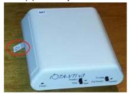
On delivery of a new IOTA-VTI, there will be insulation tag fitted to prevent battery use during shipment.
