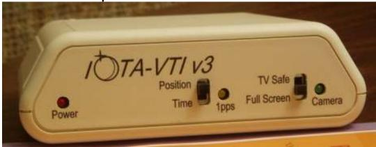
The front panel of the enclosure has two slide switches and three indicator LEDs:-
