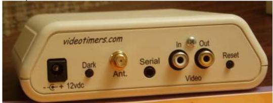
The rear panel has; a socket for Power, a Dark pushbutton, External GPS Antenna, a connector for a FTDI serial dongle, and Video In/Out, and a Reset pushbutton:-
